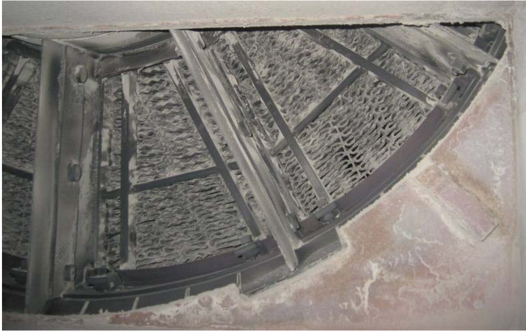
Figure 6a: Pilot Air Preheater Cold-End Basket Flue Gas Exit without \text{Mg}(\text{OH})_2 Injection
