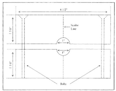
Figure 2F-6. Rotational position collar block.
