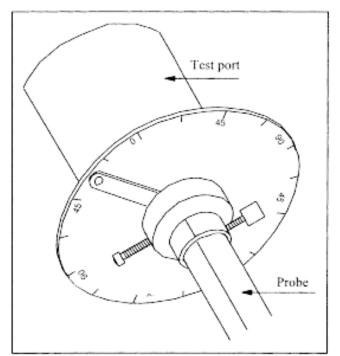
Figure 2F-7. Yaw angle protractor wheel and pointer.
