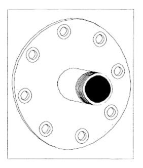
Figure 2F-5. Example bushing sleeve.
