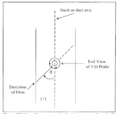
Figure 2F-10. Sign convention for the measured angle  $(\theta)$ when the probe impact port is pointed directly into the flow. The angle  $\theta$  is positive when the probe's impact pressure port is oriented in a clockwise rotational position relative to the stack or duct axis, as shown above and negative for a counterclockwise orientation.
