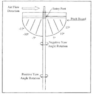
Figure 2F-8. Pitch angle protractor plate.
