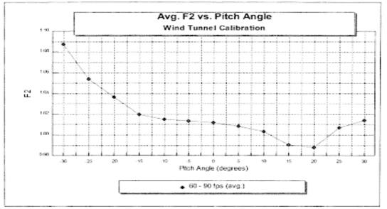
Figure 2F-15. Example F<sub>2</sub> calibration curve for the DAT probe.
