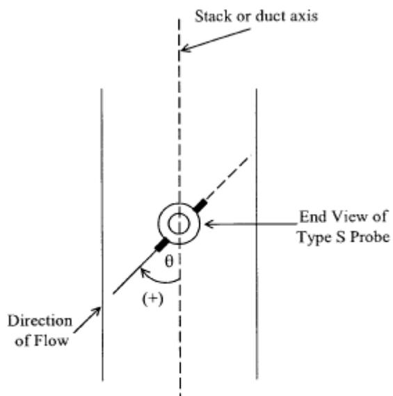
**Figure 2G-7.** Sign convention for the measured angle ( $\theta$ ) when the probe impact port is pointed directly into the flow. The angle  $\theta$  is positive when the probe's impact pressure port is oriented in a clockwise rotational position relative to the stack or duct axis, as shown above, and negative for a counter-clockwise orientation.
