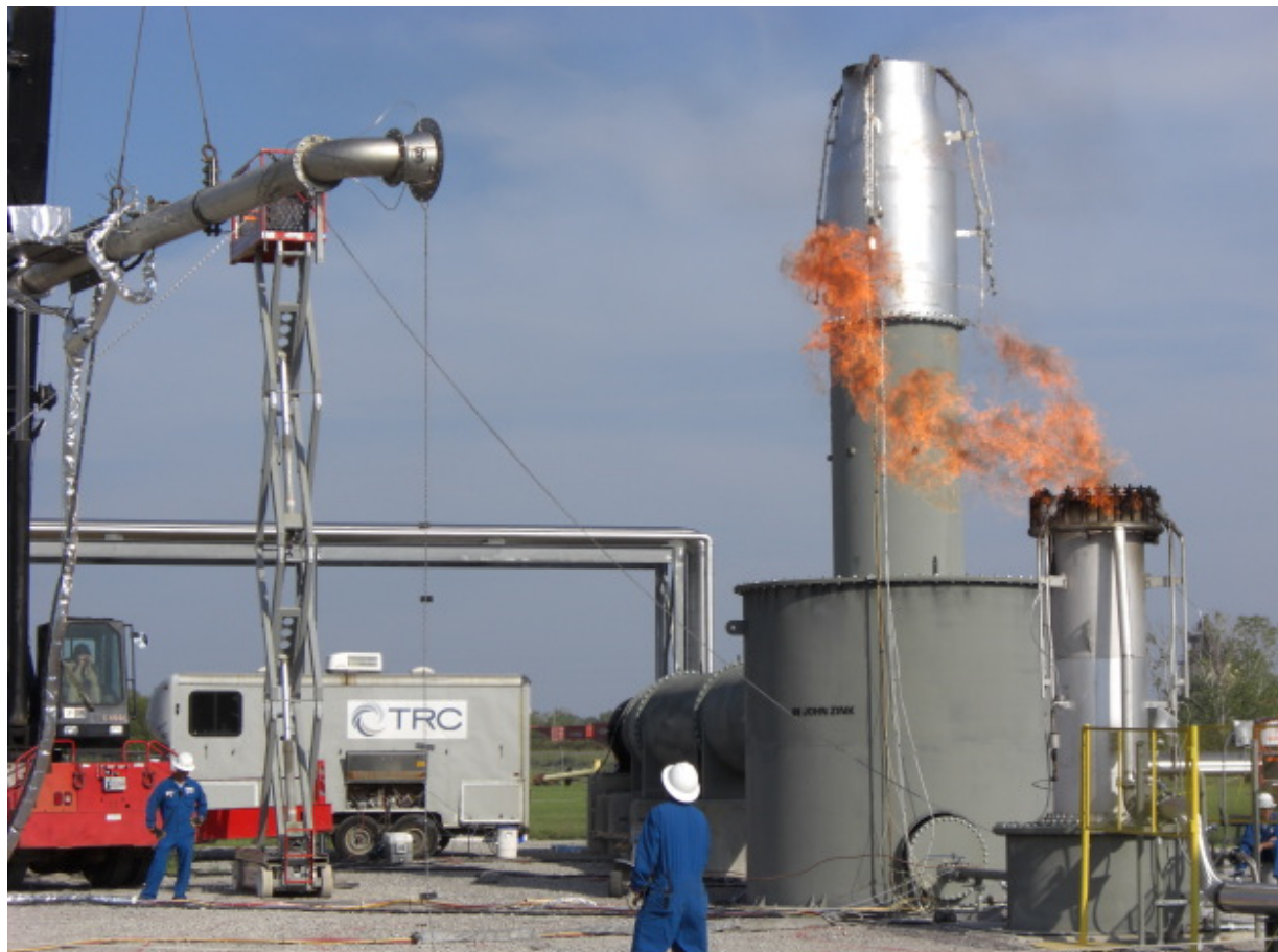
Figure ES-1. Flare Plume Sampling System. Flare Plume Sampling System making measurements of flare plume from the steam assist flare while the sampling system is held in position by crane and ground crew [4-7]*
